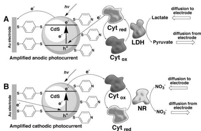
**Scheme 2** Photoelectrochemical systems composed of a monolayer of CdS NPs, soluble Cyt *c* and the respective biocatalytic systems: (A) amplified anodic photocurrent generation in the presence of reduced Cyt *c*, LDH and lactate; (B) amplified cathodic photocurrent generation in the presence of oxidized Cyt *c*, NR and nitrate.
