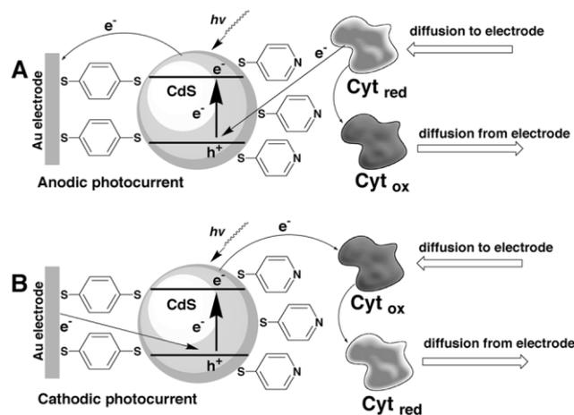
**Scheme 1** Photoelectrochemical systems composed of a monolayer of CdS NPs and soluble Cyt *c*. (A) Anodic photocurrent generation in the presence of reduced Cyt *c*. (B) Cathodic photocurrent generation in the presence of oxidized Cyt *c*.
